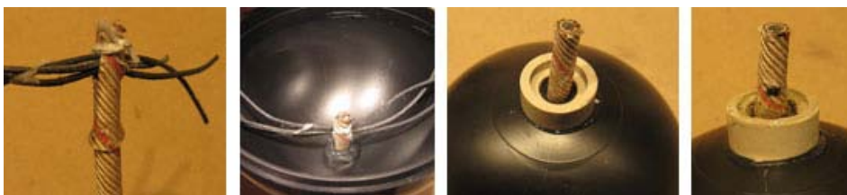
Time Fuse Hot-Glued into Shell Casing, and Sealed Inside and Out
