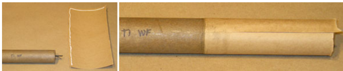
Installing Paper Buckets on Gerbs
