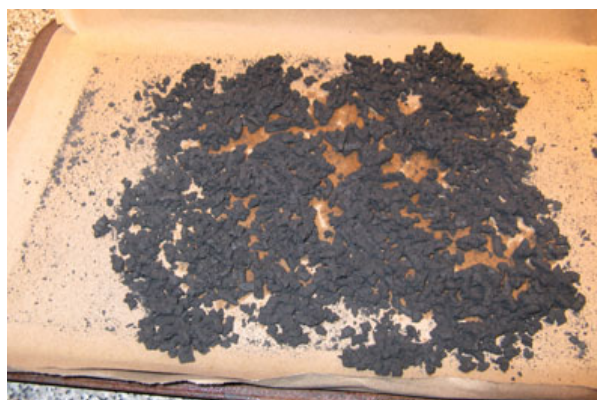
Black Powder with Red Gum and Alcohol, Granulated
