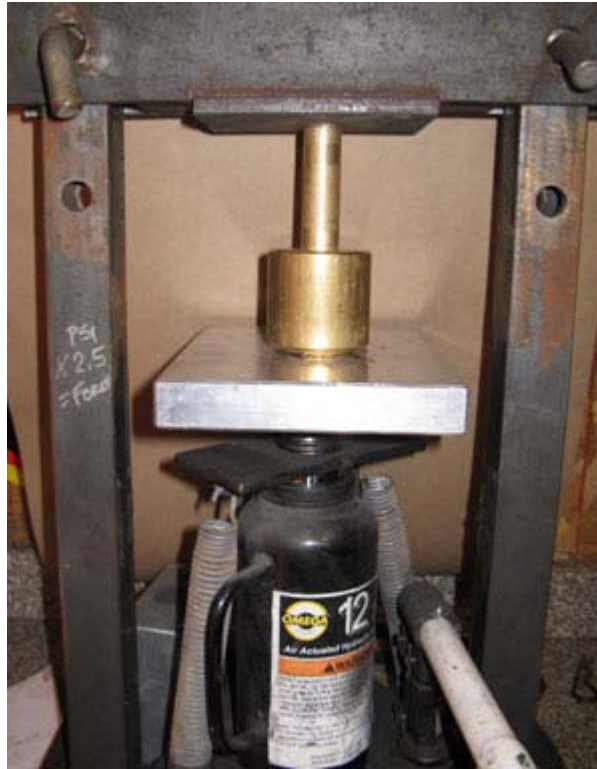
Pressing Pucks with a Hydraulic Press
