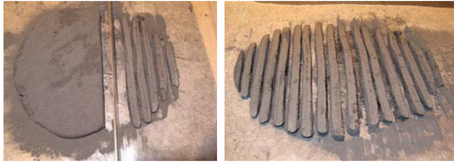
Cutting the Pancake into Strips, and Flipping Them Over
