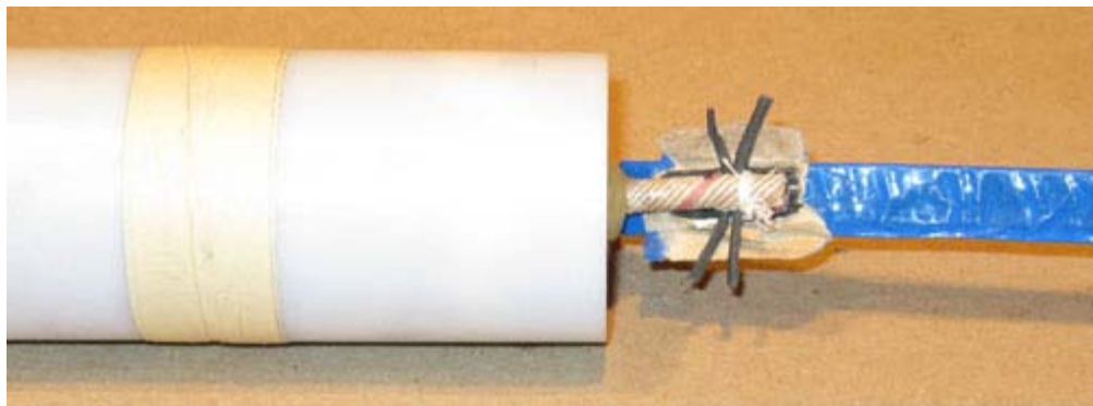
Passfire "Window" in Quick Match Leader at Upper Shell's Time Fuse
