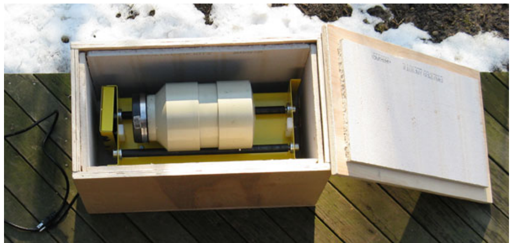
Completed Cabinet with Ball Mill Installed
