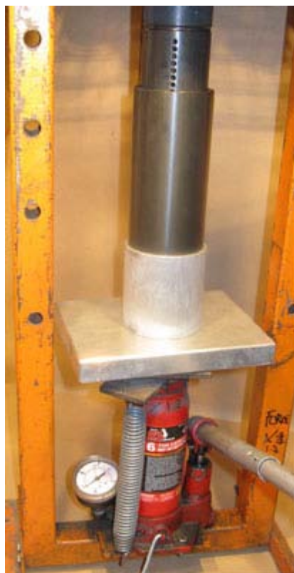
Using an Extraction-Sleeve to Push a Comet Out of the Pump
