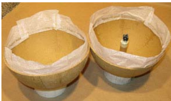
Tissue Paper Bands Hot-Glued at the Equators of Each Hemisphere
