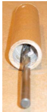
Hand-Twist-Drilling Passfire Hole through Clay Bulkhead
