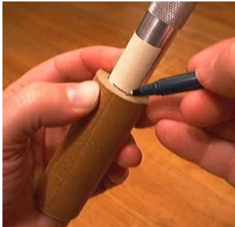
Marking Rammer for Side Vent Hole Position
