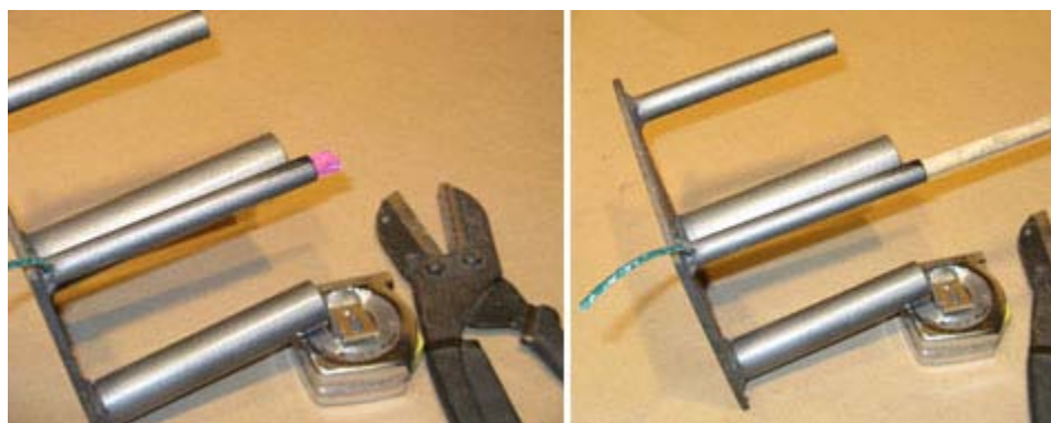
Cutting Flying-Fish Fuse and Inserting It into Tube with Dowel
