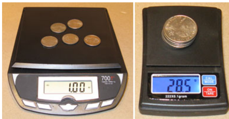
Testing the Accuracy of Digital Scales Using Five 25-Cent Pieces
