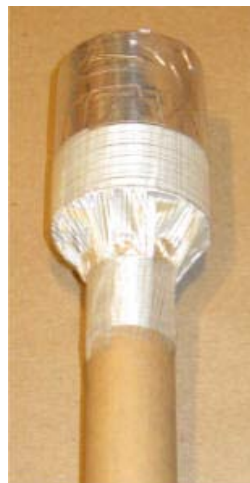
Final Heading Connection Reinforcement
