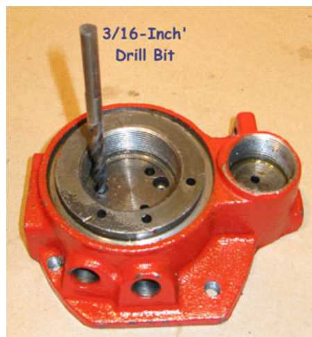
3/16-Inch Hole Drilled Down into Jack Base, Only 3/8-Inch Deep
