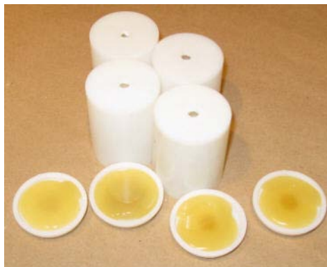
1/4-Inch Holes Drilled in Plastic Can Bottoms, Recessed Caps Filled with Hot Glue
