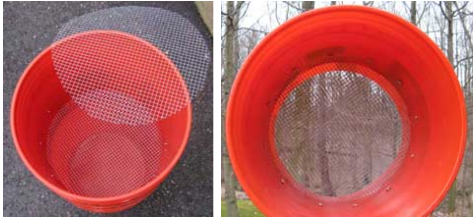
Cutting the Reinforcing Screen and Locking It into Place
