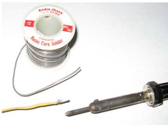
Soldering Wires onto Electric Match Head
