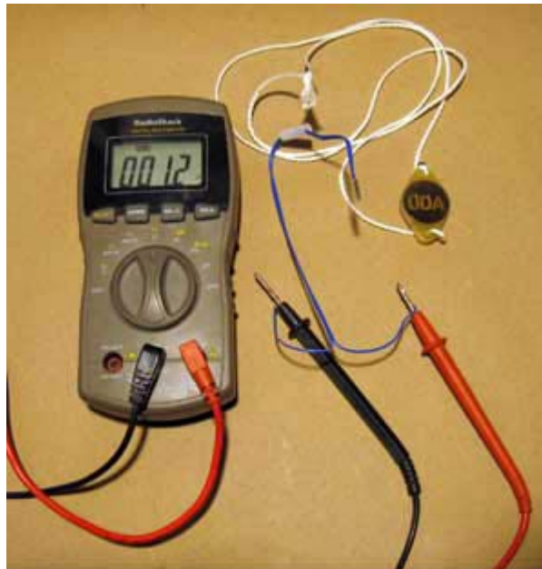
Testing Ematch Blanks with Tester and with Digital Meter
