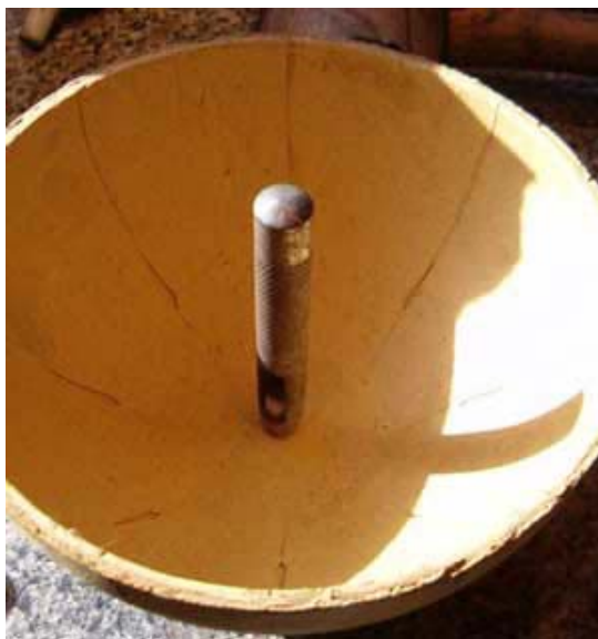
Punching Hole in Shell Casing
