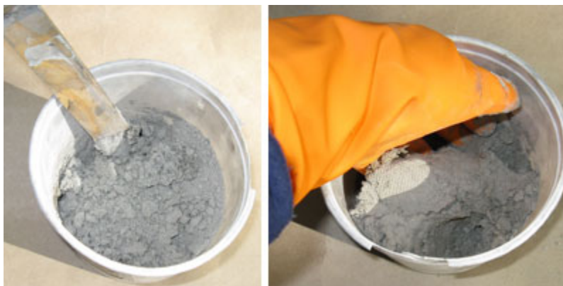
Mixing Nitrocellulose Lacquer into Strobe-Pot Composition
