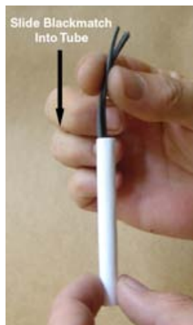
Insert Black Match into Tube
