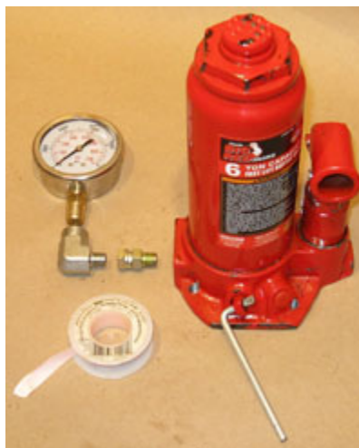
Pressure Gauge, Hydraulic Fittings, and Teflon Tape, Ready to Be Installed on Bottle Jack
