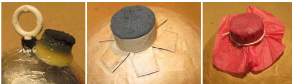
Attaching Comet to a Aerial Shell for Rising Tail Effect
