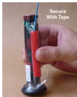
Tape Electric Match in Place
