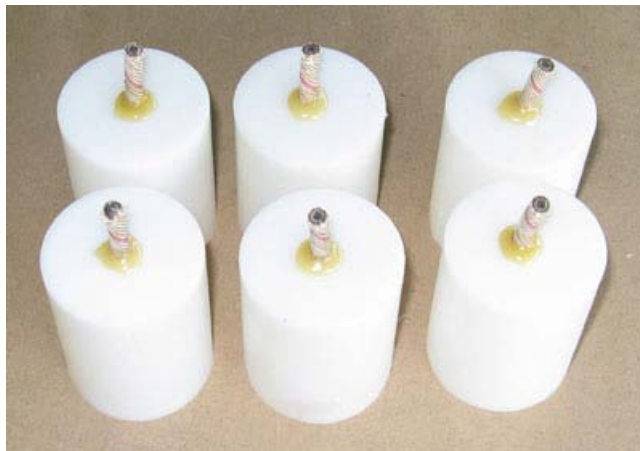
Time Fuses Sealed on the Outside of the Plastic Shell Caps
