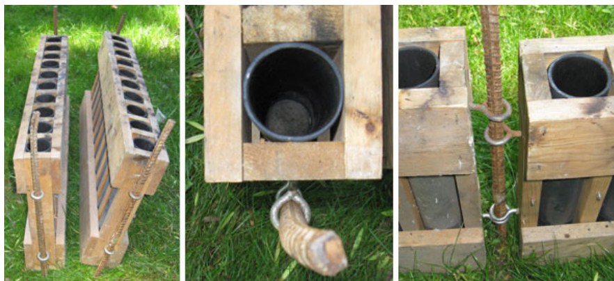
Wooden Racks Secured with Screw-Eyes and Rebar Pins
