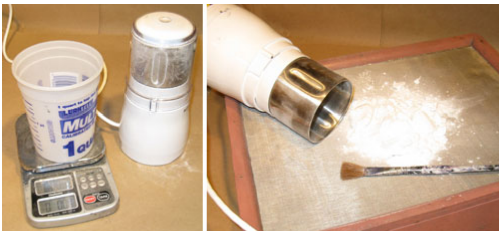
Successfully Milling Potassium Nitrate with a Coffee Blade Grinder
