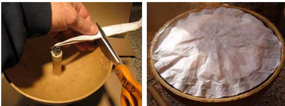
Shell Hemi Sealed with Disc of Tissue Paper, Hot-Glued in
