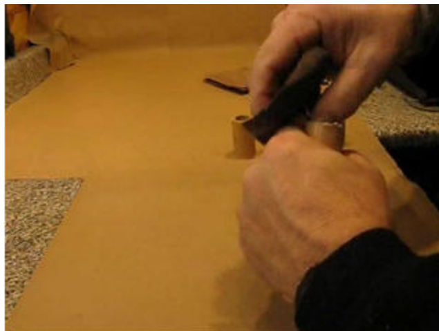
Sanding Ends of Roman Candle Tube Sections
