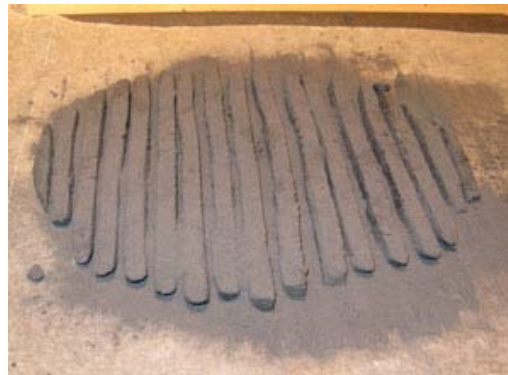
Strips of Star Comp Dusted on Both Sides with Black Powder Prime
