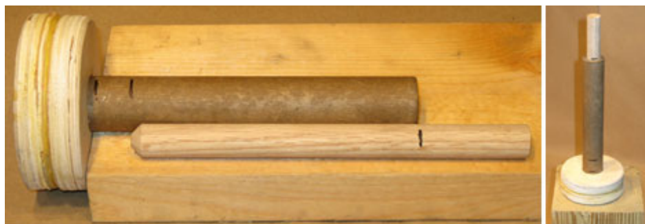
Marking the Nozzle Rammer, and Ramming Clay to Form Nozzle
