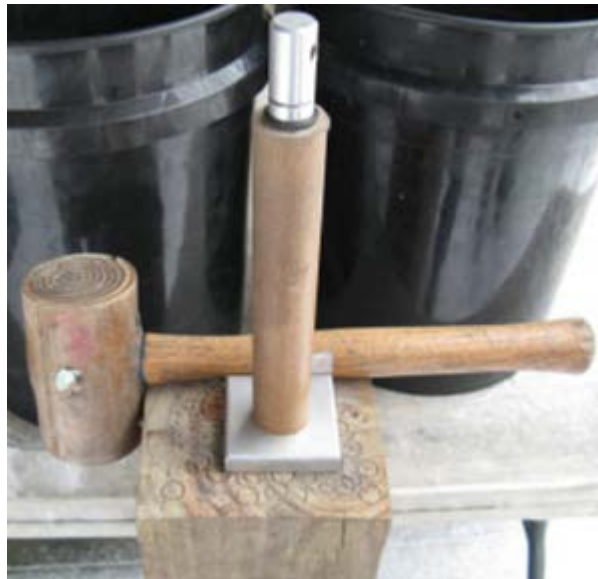
Ram Mix into Tube with Nozzle Forming Tool and Mallet
