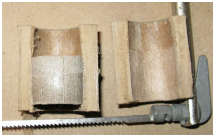
Cutaway Paper Tube Showing Locked-In Clay Bulkhead
