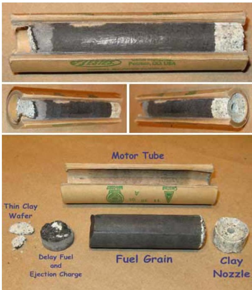
A Dissected Estes E9-6 Model Rocket Engine
