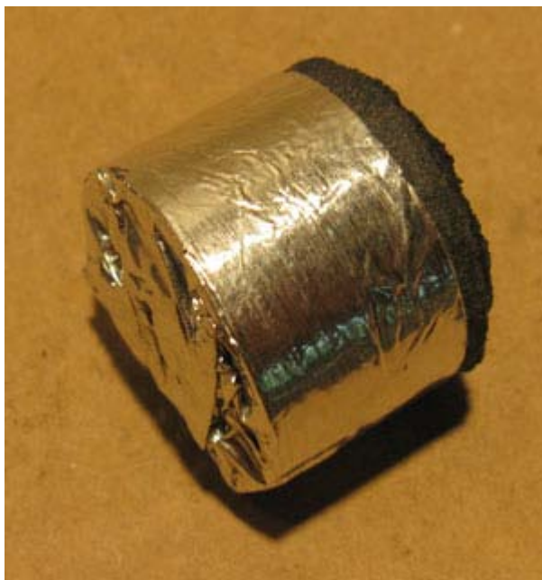
Foil-Tape-Wrapped Comet Ready to be Fired and Timed
