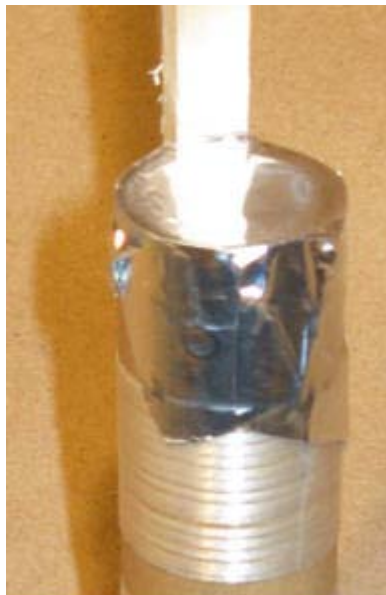
Sealing Bottom of Rocket Motor and Fuse-Hole with Aluminum-Foil Tape
