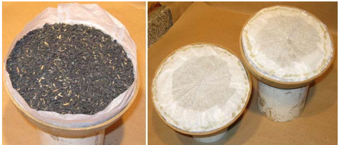
Black-Powder-Coated Rice Hulls Filled in around Blue Stars, Both Hemispheres Capped and Ready to be Mated
