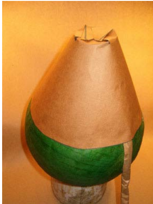
Lift Cup, Covering Lift Powder, Glued to Shell
