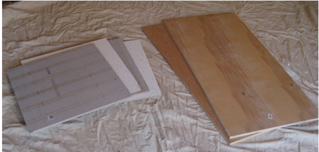
Ceiling Tiles for Sound Insulation and Plywood
