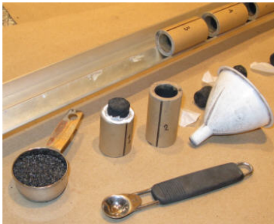
First Roman Candle Section--Loaded with Lift Powder, Tissue Paper Disk and Star, Elmer's Glue Applied
