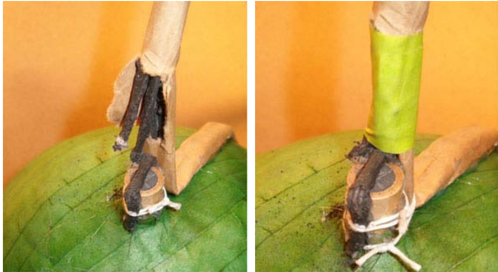
Shell Leader and Spolette Match Joined and Secured
