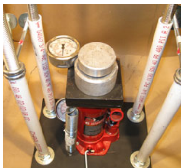
A Pressure-to-Force Gauge Being Used with the Hydraulic Press
