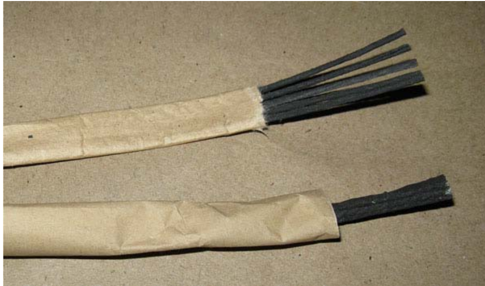
Black Match and Paper Match Pipe Combine to Make Quick Match
