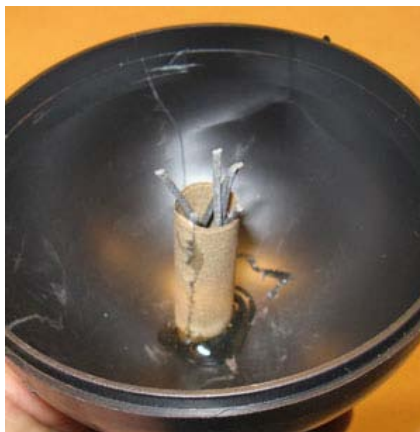
Passfire Tube Hot-Glued into Shell Casing
