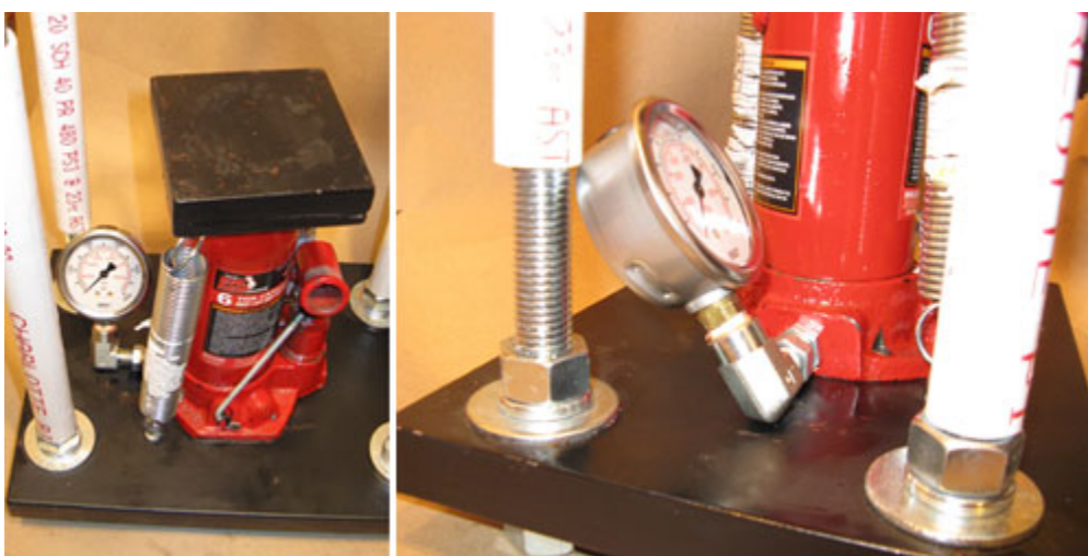
Hydraulic Bottle Jack with Gauge, Installed on Rocket Press
