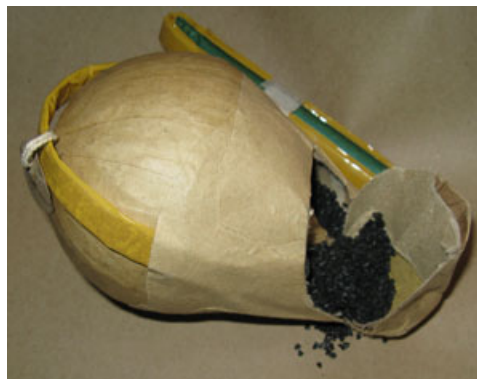
Black Powder Used as Shell Lift Powder
