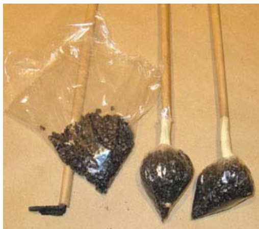
Black Powder Lift Charge, Baggie, and Quick Match Fuse Leader
