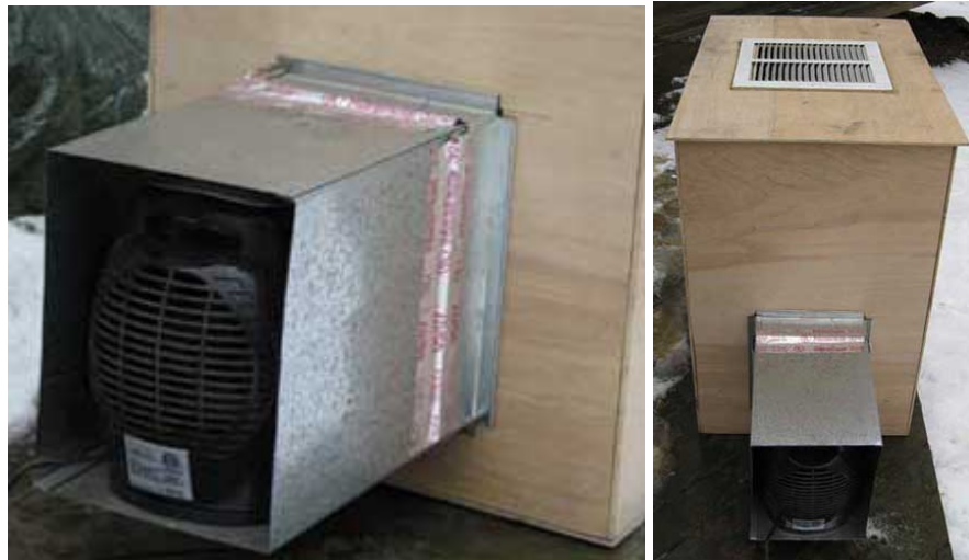
Heater, Duct, and Cover Detail of Drying Chamber
