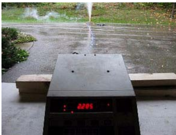
Estes E9-4 Rocket Engine's Thrust Measured with a Digital Scale
