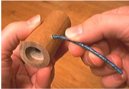
Installing Fuse in Side Vent Hole
