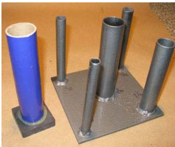
Mortar and Star Gun Used to Test-Fire Glitter Comets
