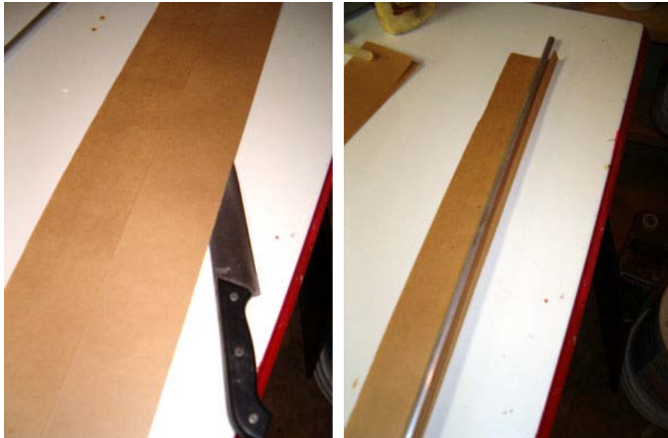
Cutting Kraft Paper and Rolling It around an Aluminum Rod
