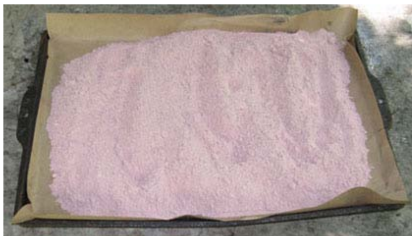
Screened Whistle Mix Drying on Kraft-Paper Lined Tray
