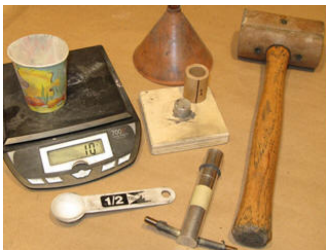
Ramming Clay Plug into Roman Candle Bottom Section
