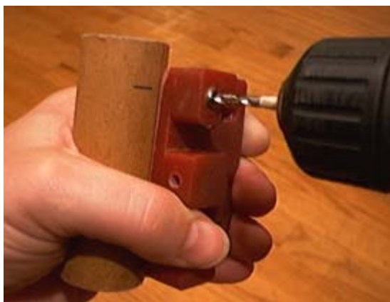
Drilling Side Vent Hole in Tube
