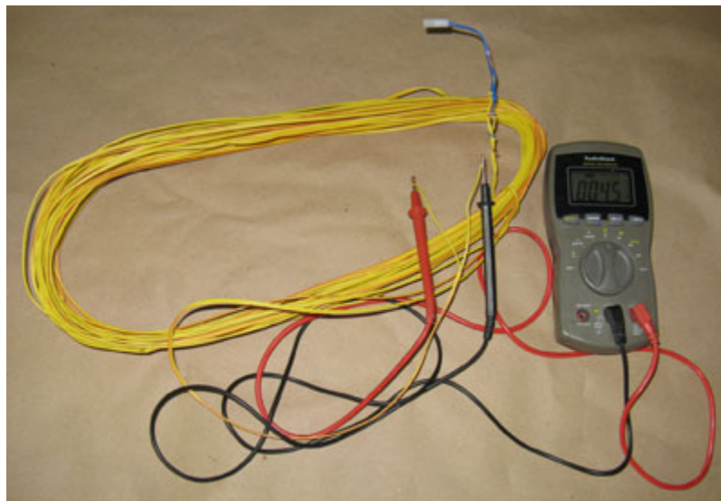
Ematch and 100 Feet of Shooting Wire, Reading 4.5 Ohms
