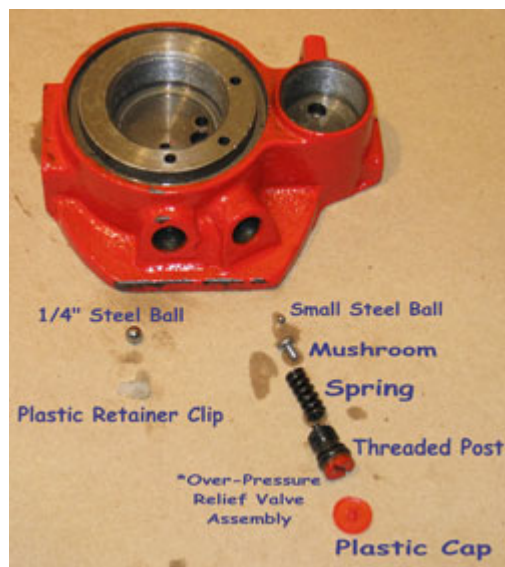
Final Bottle-Jack Disassembly
