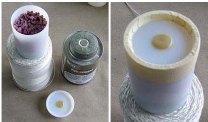
Cap of Plastic Shell Casing Glued and Taped in Place
