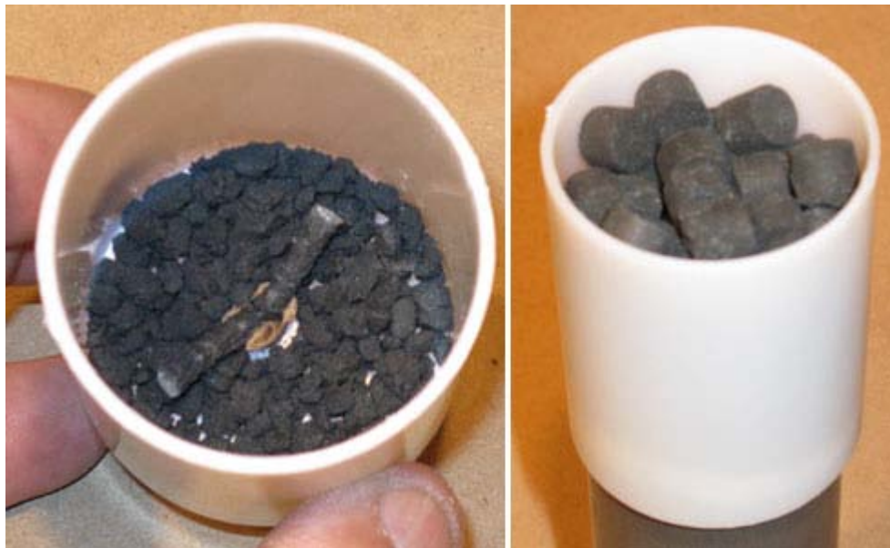
Black Powder, Tissue Paper, and Stars Placed in Shell Casing
