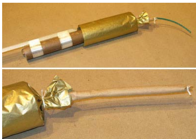
Loose Protective Wrapping Installed Over Comet, Visco Fuse and Safety Cap Installed
