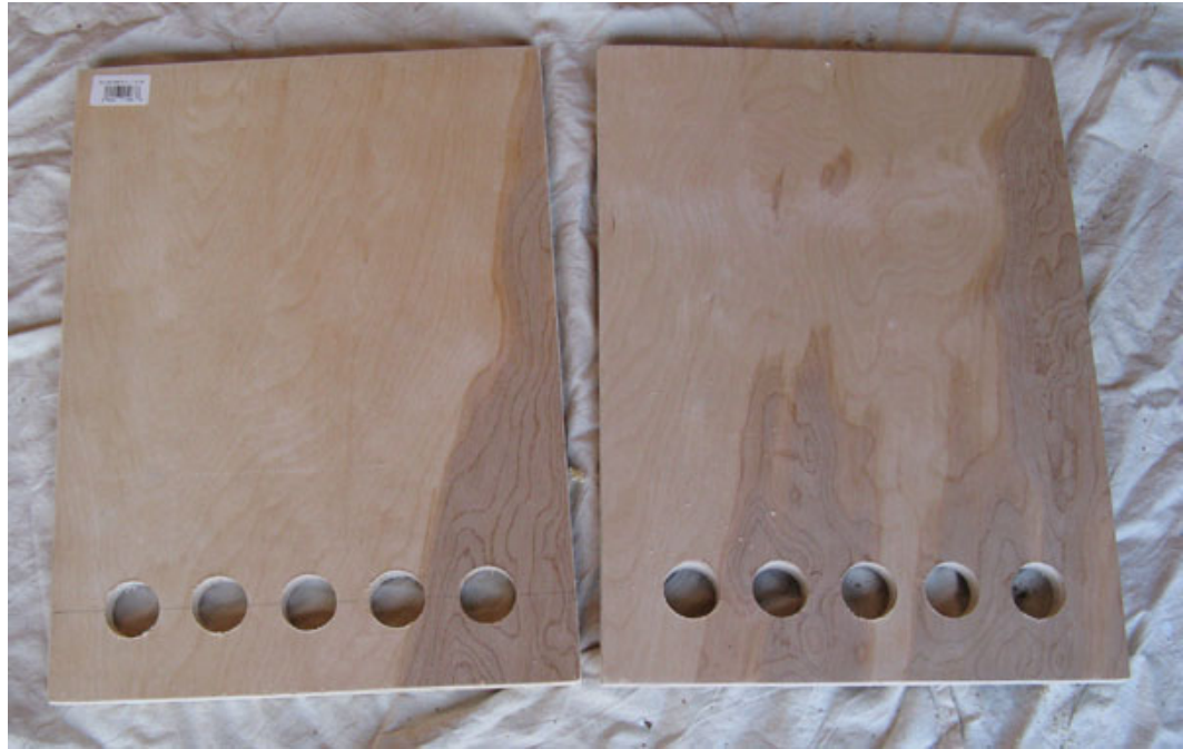
Ventilation Holes Drilled in Cabinet Sides
