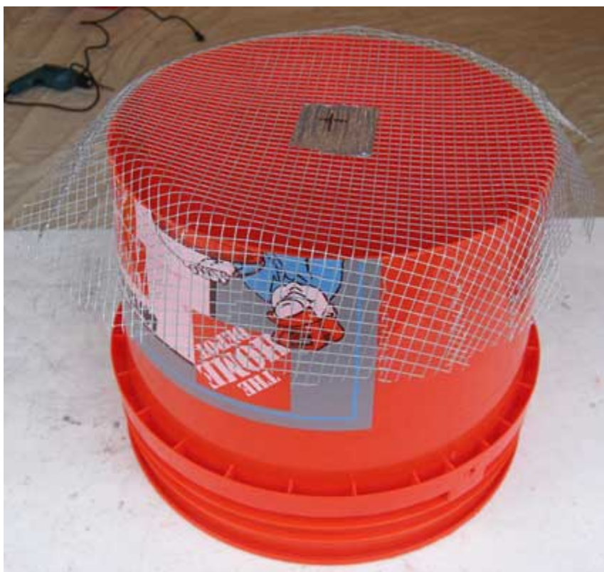
Screen Folded onto One 9-1/2" Deep Bucket
