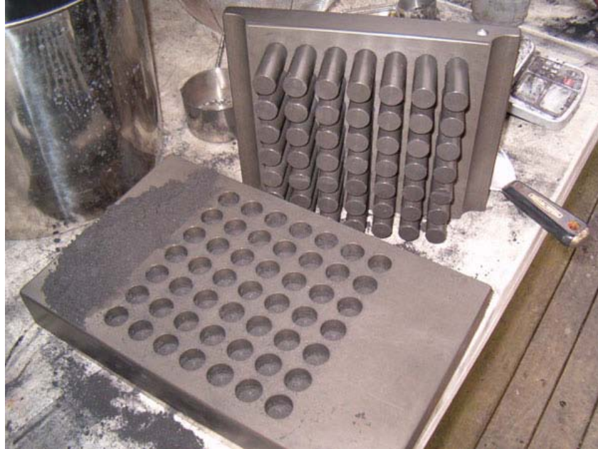
Loading Composition into Star Plate
