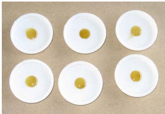
Recesses in Shell Casing Caps Filled with Hot-Glue
