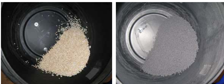
Coating BP onto Puffed Rice in Star Roller
