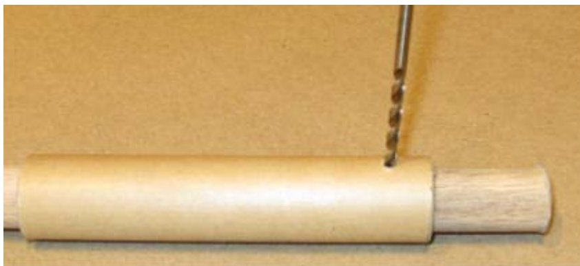
Drilling 1/8-Inch Fuse Hole in Whistle-Rocket Motor Tube
