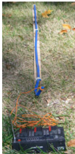
Three Strobe Pots Ready to Be Electrically Fired
