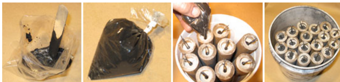
Priming the Gerbs with Black Powder Slurry
