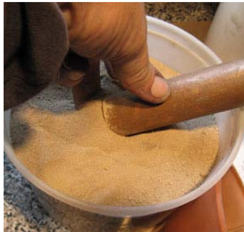
Inserting Clay into Tube, and Clay Bulkhead Mix Rammed in Tube
