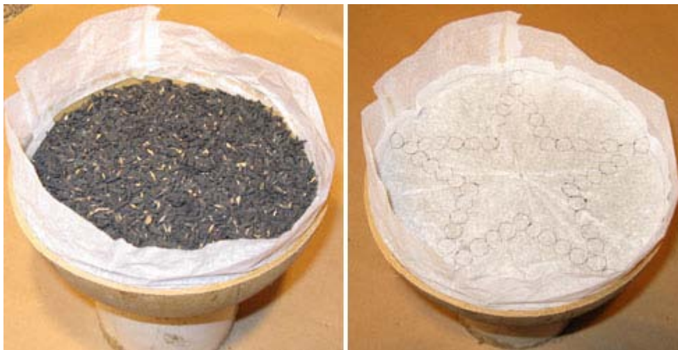
Second Shell Hemisphere Filled to Within 3/8 Inch of Rim, and Capped with Star Patterned Tissue Paper Disc
