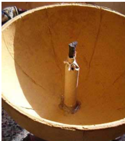
Black Match and Passfire Tube Installed, with Vent Hole
