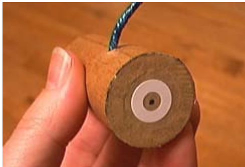
Reinforced Exhaust Hole
