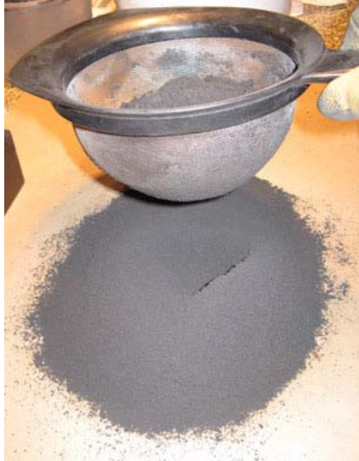
Screening Black Powder to Incorporate Water
