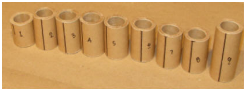
Roman Candle Tube Cut into Sections
