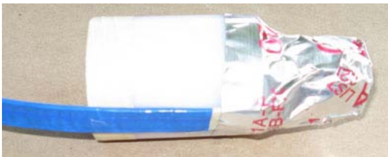
Bottom of Shell Covered with Aluminum-Foil Duct Tape
