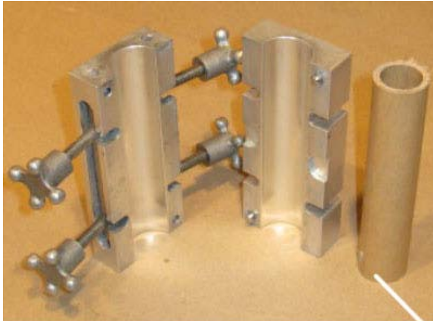
Clamshell Support for Pressing Whistle in Paper Tubes
