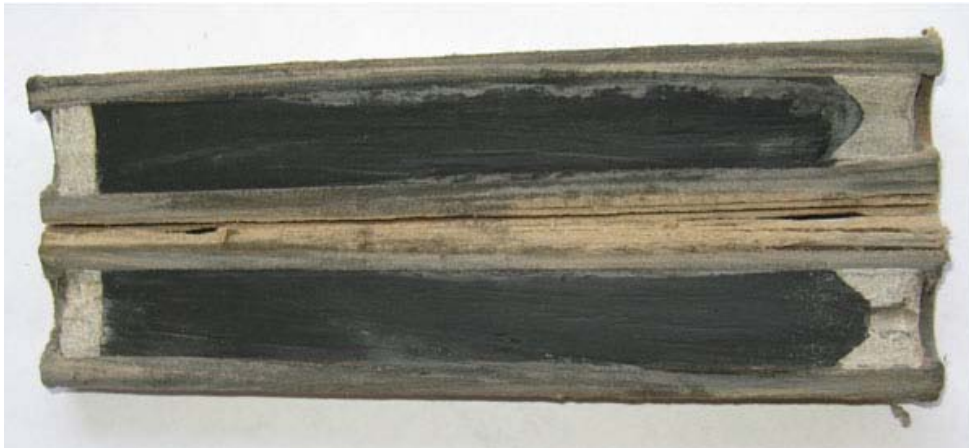
End Burner Rocket Motor
