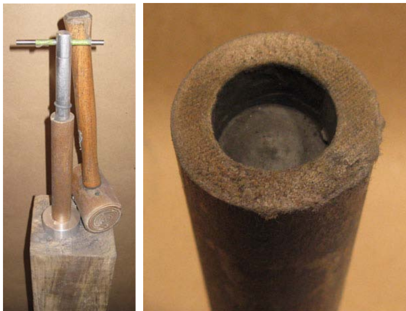
Ramming Fuel in Tube
