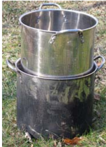
Pot Containing Whistle Mix Drying in Hot-Water Bath
