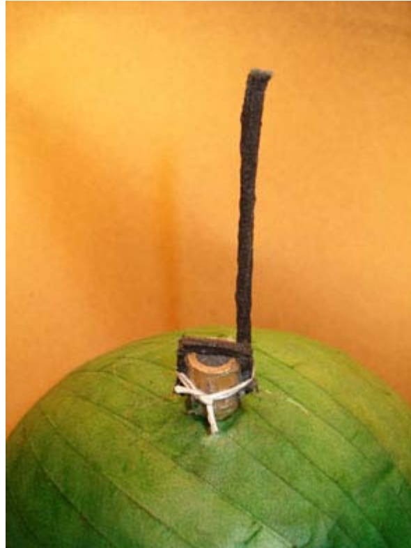
Black Match Hot-Glued and Tied to Spolette, after Scratching BP
