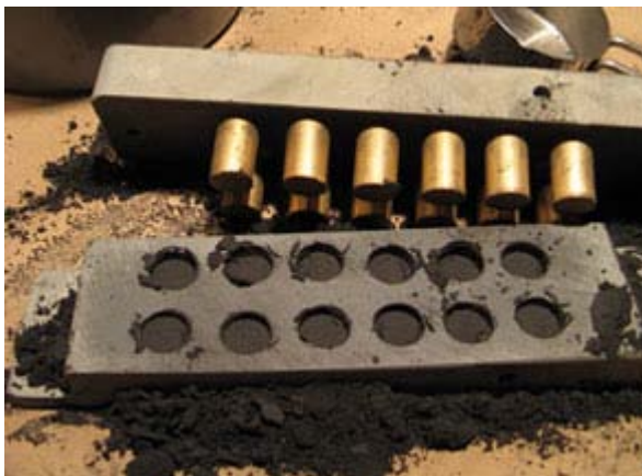
Loading Star Plate with Comp
