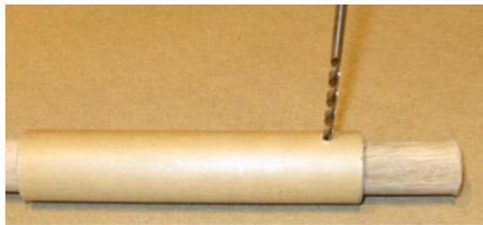
Drilling Fuse Hole in Strobe-Rocket Tube
